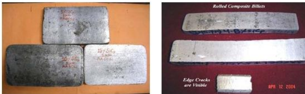
Fig 4: As-cast Composite Rolled Billets
