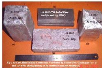
Fig 3: shows as-cast MMC in different mould shapes to facilitate
