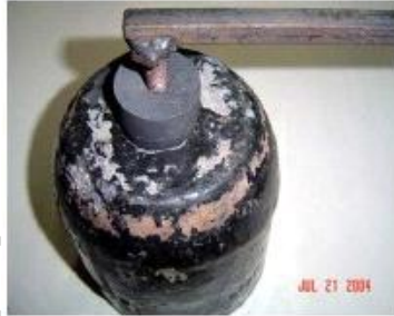
Fig 1(c): Shows Bottom pour facility in SiC crucible
