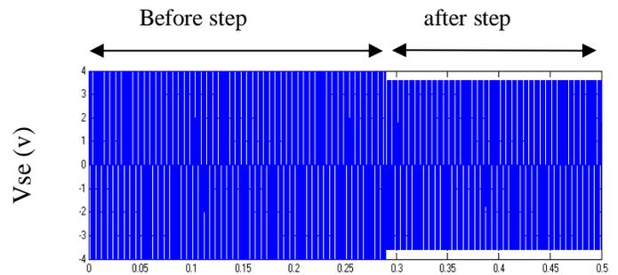
Fig.no.13. Step response of the DPFC: Series Converter voltage.
