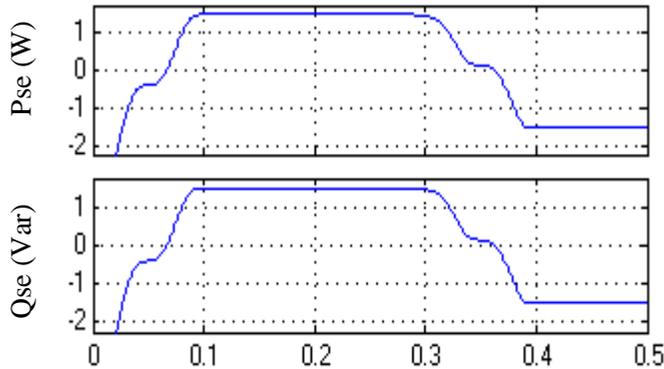
Fig.no.14. Active and reactive power injected by the series converter at the fundamental frequency.
