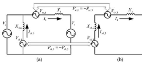
Fig.no.6. DPFC equivalent circuit (a) Fundamental frequency (b) Third-harmonic frequency.
