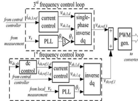
Fig.no.9. Block diagram of the shunt converter control.
