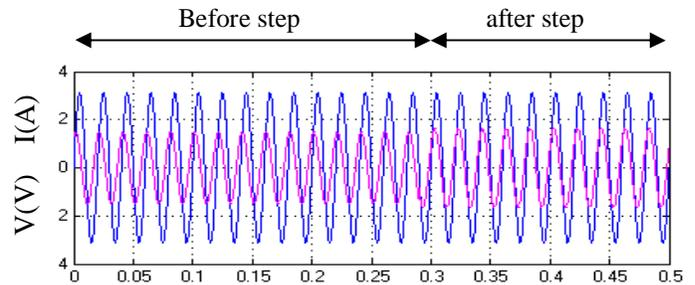
Fig.no.12. Step response of the DPFC: Bus voltage and current at the  $\Delta$  side of the transformer.
