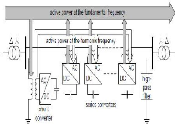
Fig.no.2. Active power exchange between DPFC converters
