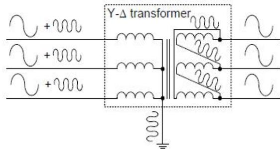
Fig.no.3. Utilize grounded Y- $\Delta$  transformer to provide the path for the zero sequence third harmonic.
