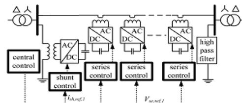
Fig.no.7. DPFC control block diagram.
