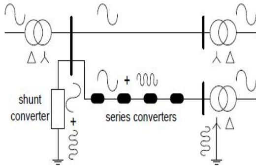
Fig.no.4. Route the harmonic current by using the grounding status of the Y-Δ transformer.
