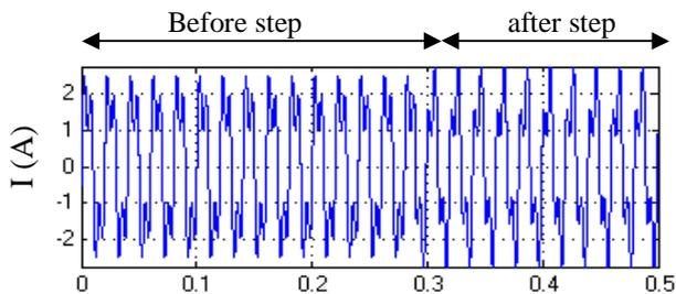
Fig.no.11. Step response of the DPFC: line current.
