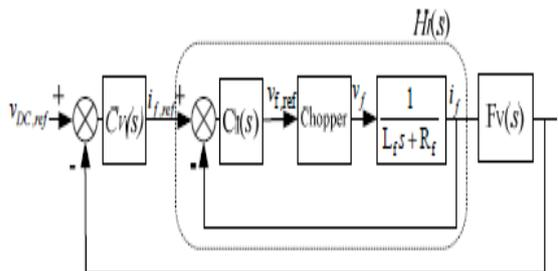
Fig.4 Block diagram of the voltage regulation
