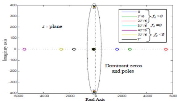
Fig.6 Poles and zeros map of  $Gv(s)$  for different values of  $(fd, fq)$
