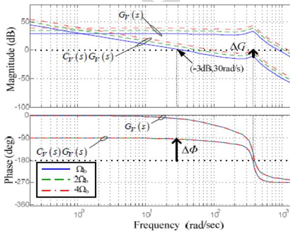
**Fig.8** Bode plots of  $G_v(s)$  and  $C_v(s) G_v(s)$  for different rotor speeds
