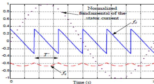
Fig.5  $fd(t)$  and  $fd(t)$  waveforms on a period of the stator current
