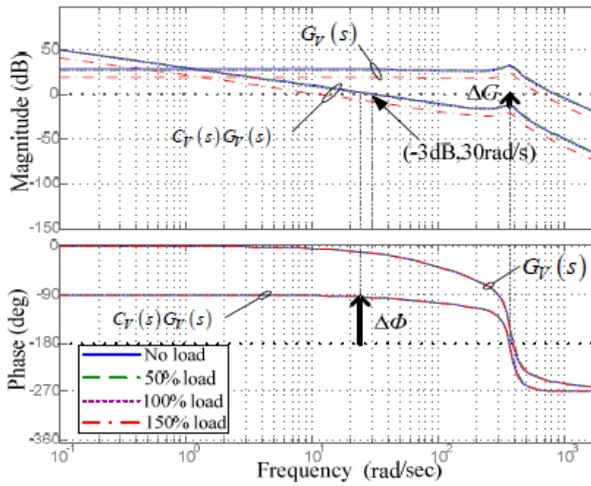
**Fig.7** Bode plots of  $G_v(s)$  and  $C_v(s) G_v(s)$  for different loads
