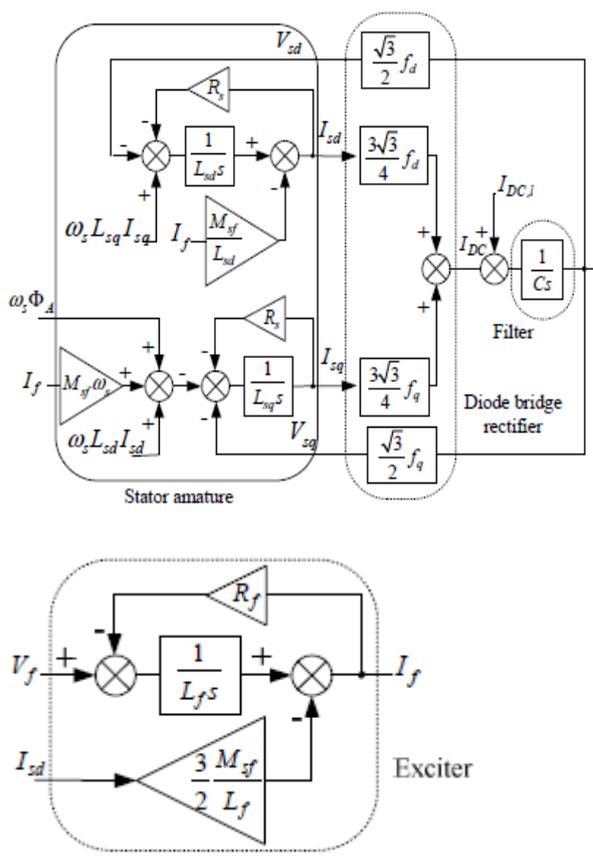
Fig.2 DC Generator block diagrams
