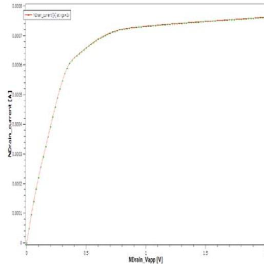
Figure 8:  $I_D$  versus  $V_{DS}$  at  $V_{GS}=2V$
