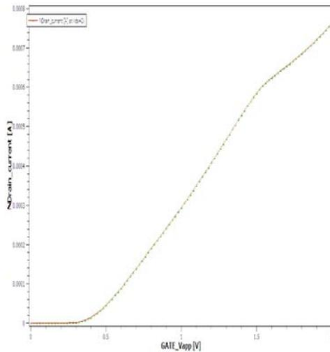
Figure 7:  $I_D$  versus  $V_{GS}$  at  $V_{DS}=2V$
