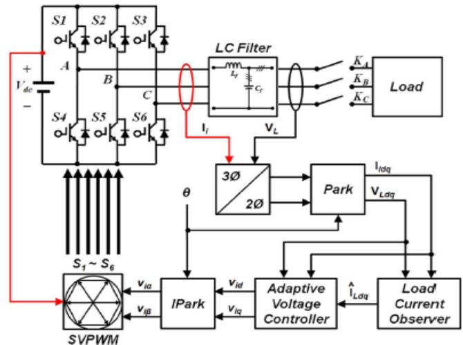
Fig.5. Overall block diagram of the proposed adaptive control system.
