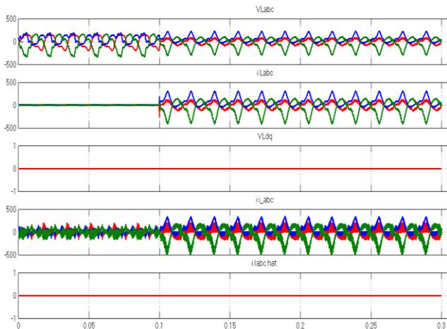
Fig.7. Simulation results without the proposed control scheme under Case 1 for a 200-kVA unit (balanced resistive load: 0%–100%).
