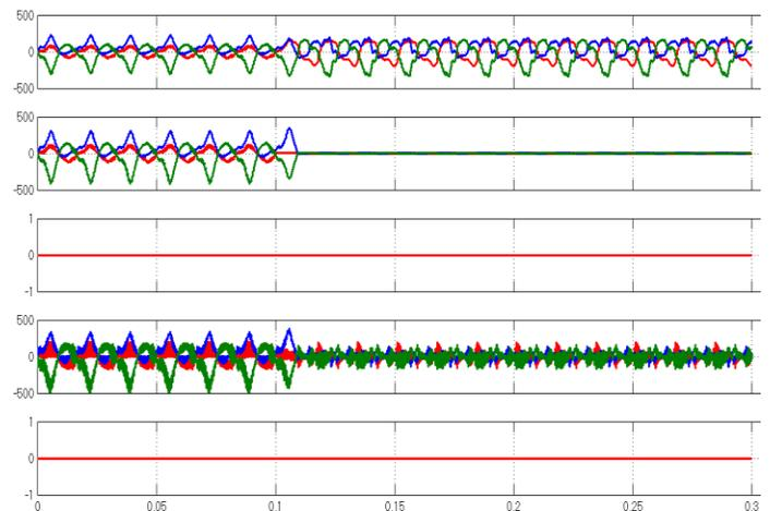
Fig.9. Simulation results without the proposed control scheme under Case 2 for a 200-kVA unit (balanced resistive load: 100% to 0%).
