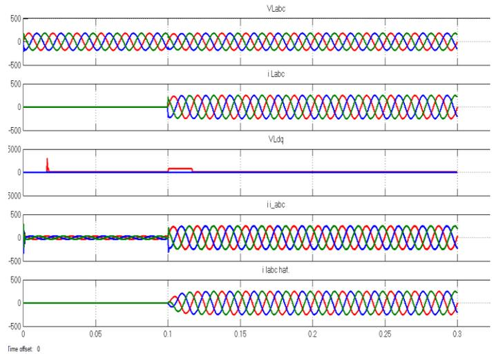
Fig.8. Simulation results of the proposed control scheme under Case 1 for a 200-kVA unit (balanced resistive load: 0%–100%).
