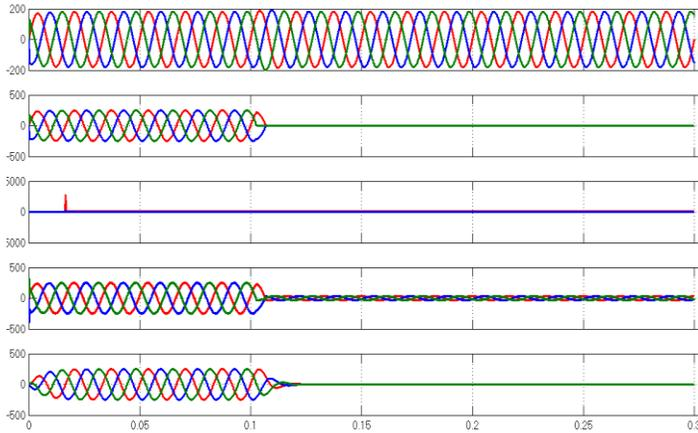
Fig.10. Simulation results of the proposed control scheme under Case 2 for a 200-kVA unit (balanced resistive load: 100% to 0%).
