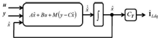
Fig.4. Block diagram of the proposed optimal load current observer.
