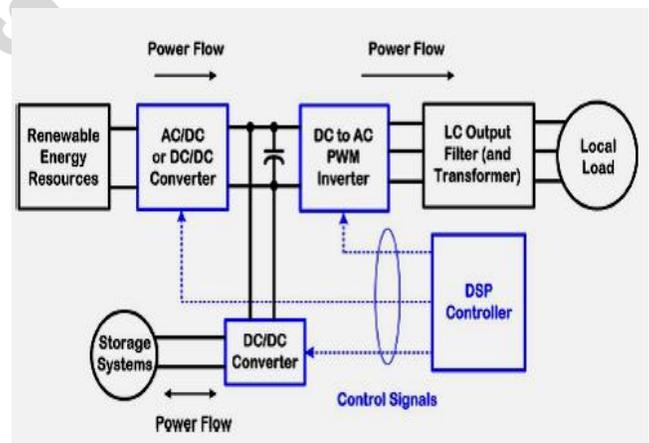
Fig.1. Configuration of a typical DGS in a stand-alone operation.
