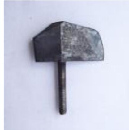
Eroded Jet Vane at  $\alpha = 5$  deg
