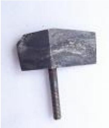
Eroded Jet Vane at  $\alpha = 0$  deg
