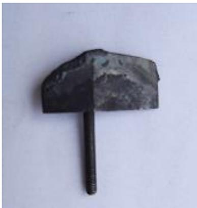
Eroded Jet Vane at  $\alpha = 10$  deg
