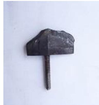
Eroded Jet Vane at  $\alpha = 15$  deg
