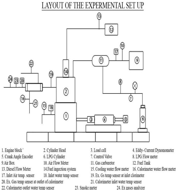
**Figure 1 Layout of the Experimental Set-up**
