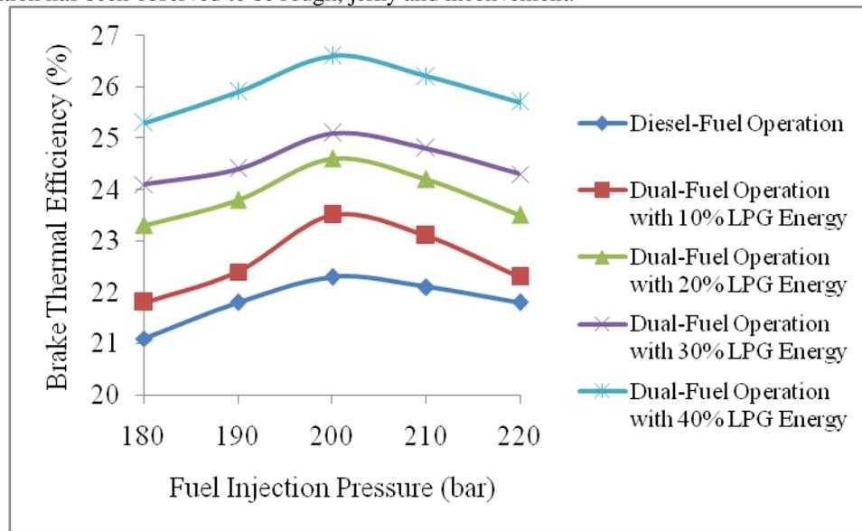
**Figure 5 Effect of Fuel Injection Pressure on the Brake Thermal Efficiency on Dual-Fuel Mode of Operation for Different Levels of Substitution of LPG at 60% Load**
