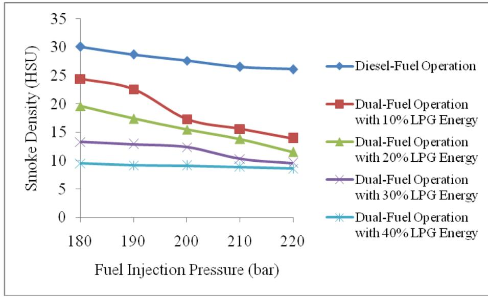
**Figure 6** Effect of Fuel Injection Pressure on the Smoke Density on Dual-Fuel Mode of Operation for Different Levels of Substitution of LPG at 60% Load
