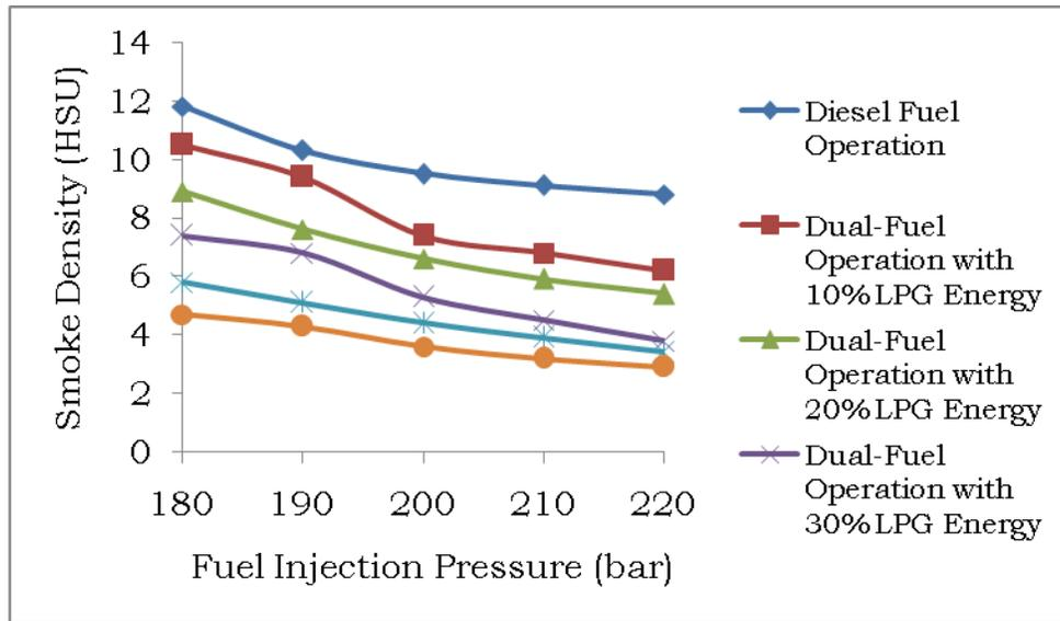
**Figure 3** Effect of Fuel Injection Pressure on the Smoke Density on Dual-Fuel Mode of Operation for Different Levels of Substitution of LPG at 20% Load
