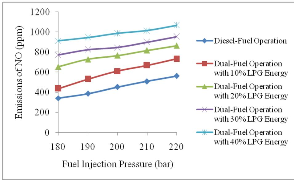
**Figure 7** Effect of Fuel Injection Pressure on the Emissions of NO on Dual-Fuel Mode of Operation for Different Levels of Substitution of LPG at 60% Load
