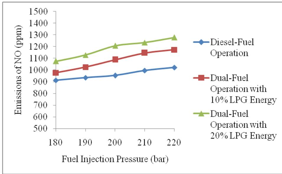
**Figure 10** Effect of Fuel Injection Pressure on the Emissions of NO on Dual-Fuel Mode of Operation for Different Levels of Substitution of LPG at 80% Load
