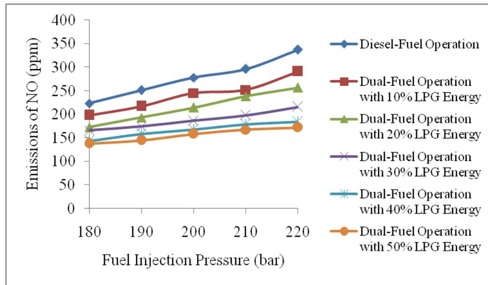
**Figure 4** Effect of Fuel Injection Pressure on the Emissions of NO on Dual-Fuel Mode of Operation for Different Levels of Substitution of LPG at 20% Load
