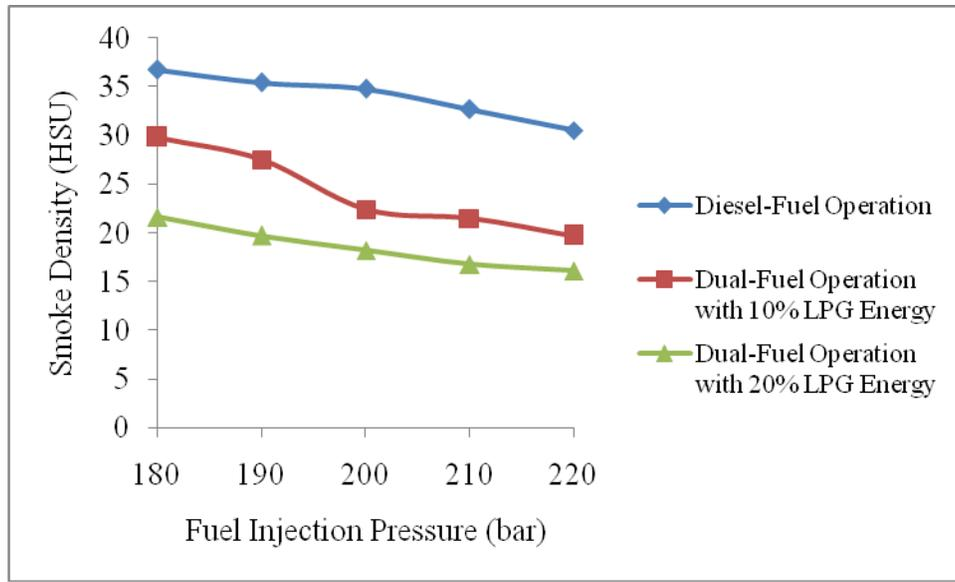
**Figure 9** Effect of Fuel Injection Pressure on the Smoke Density on Dual-Fuel Mode of Operation for Different Levels of Substitution of LPG at 80% Load
