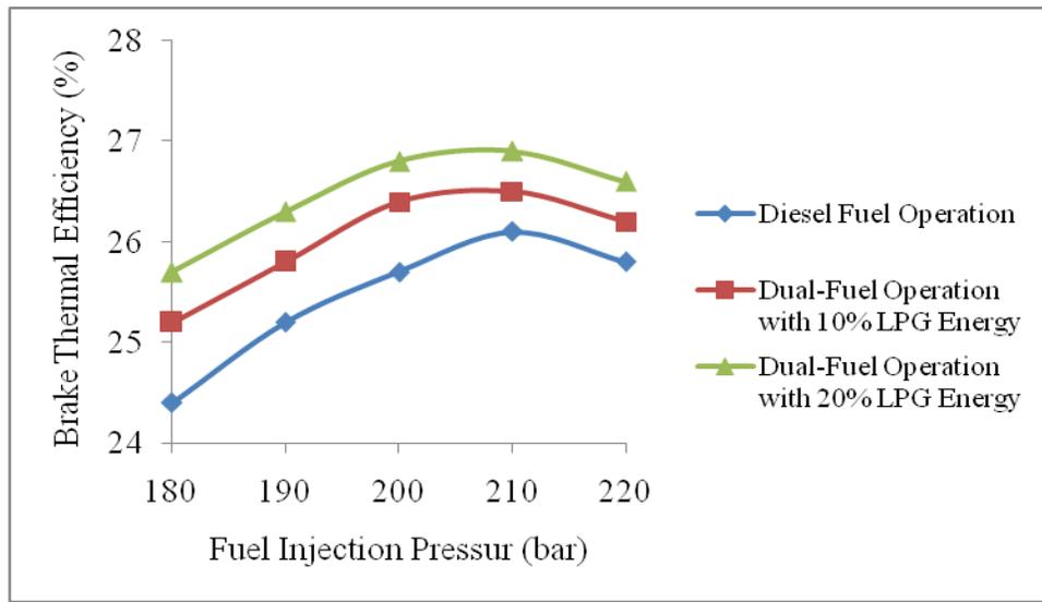
**Figure 8** Effect of Fuel Injection Pressure on the Brake Thermal Efficiency on Dual-Fuel Mode of Operation for Different Levels of Substitution of LPG at 80% Load
