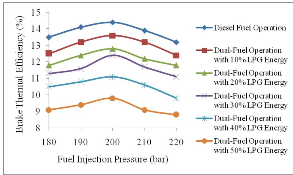
**Figure 2** Effect of Fuel Injection Pressure on the Brake Thermal Efficiency on Dual-Fuel Mode of Operation for Different Levels of Substitution of LPG at 20% Load
