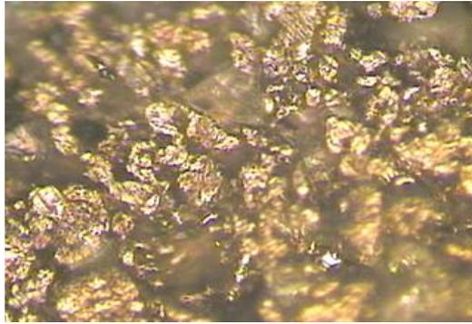
Fig.:2 Microstructure of Al-15% graphite compact edat 100 MPa sintered at 500°C - 90min.
