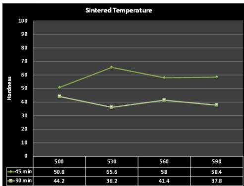
Sintered temperature Vs hardness
