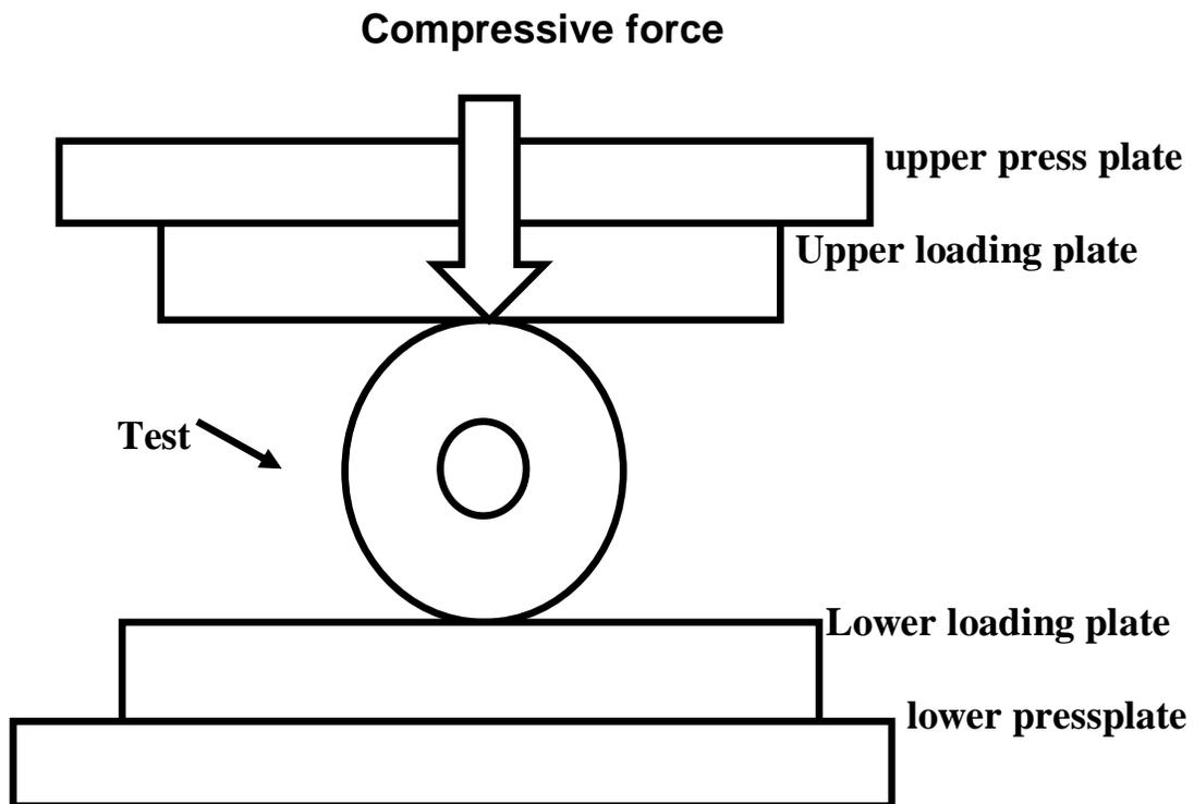
**Fig.: 2** Experimental arrangement showing the holding of the ring shaped Specimen. The Radial Crushing Strength is obtained using the formula given below.
