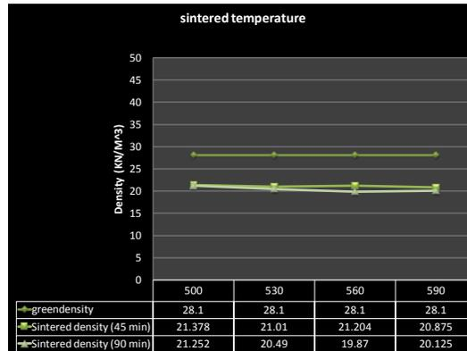
sintered temperature Vs Density
