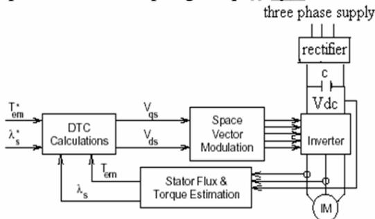
Fig 1. Block Diagram of SVM-DTC
