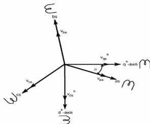
Fig 2. Stationary frame a~b~c to  $d^s$ ~ $q^s$  axes transformation
