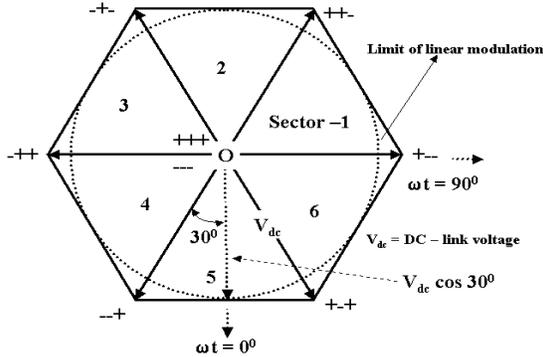
Fig 8. Determination of the sample-averaged pole voltage
