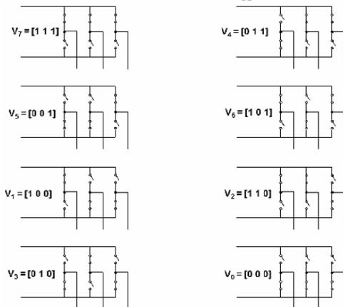
Fig 4. Eight inverter voltages vectors ( $V_0$  to  $V_7$ )
