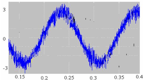
Fig 15. Stator d-current with conventional DTC
