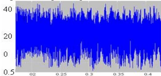
Fig 13. Out put torque with conventional DTC
