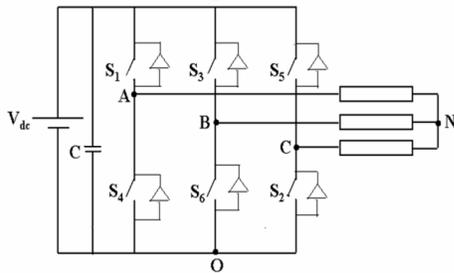
Fig 3. Power circuit of a three-phase VSI
