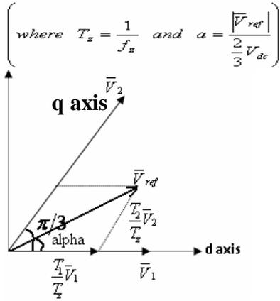
Fig 6. Reference vector as a combination of adjacent vectors at sector-1
