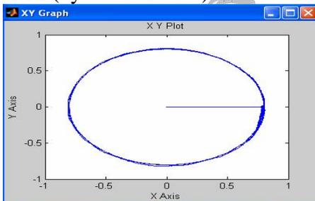
Fig 10. d-q stator flux with SVM-DTC
