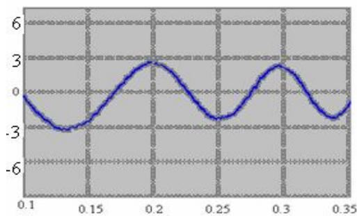
Fig 14. Stator d-current with SVM-DTC
