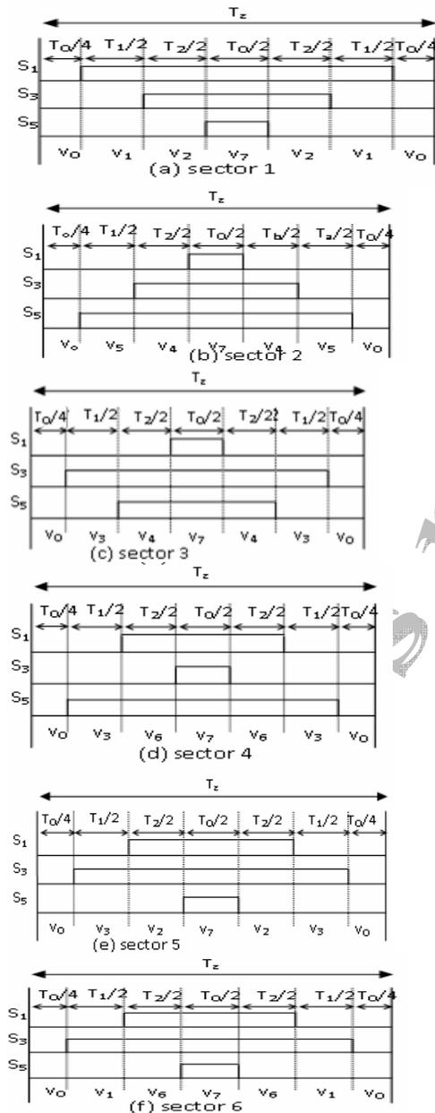
Fig 7. SVPWM switching patterns of upper switches at each sector
