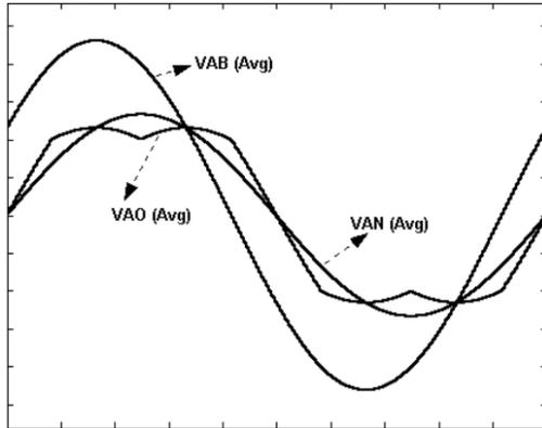
Fig 9. Waveforms of averaged pole voltage, phase voltage and line-line voltage
