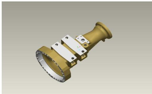
Fig 1: solid model of Rear Axle housing
