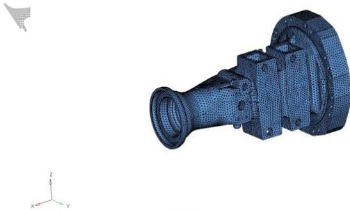
Fig 3: FE Model of Rear Axle housing
