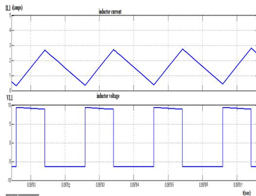
Fig.7. Inductor 1 current & voltage wave forms
