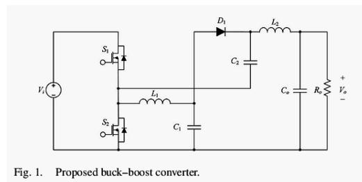
Fig. 1. Proposed buck-boost converter.
