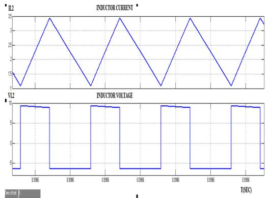
Fig.8. Inductor 2 current & voltage wave forms
