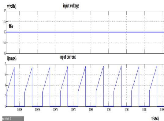
Fig.5. Input voltage & current wave forms
