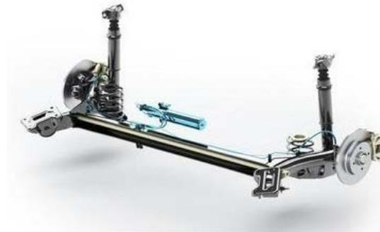
Fig. 2. ARC system of BMW using a hydraulic rotary actuator [10].
