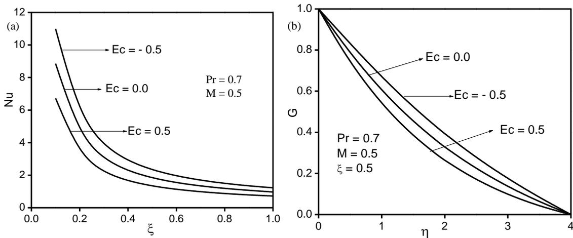
**Fig.4. Effect of viscous dissipation on (a) Heat transfer coefficient (b) Temperature profile**
