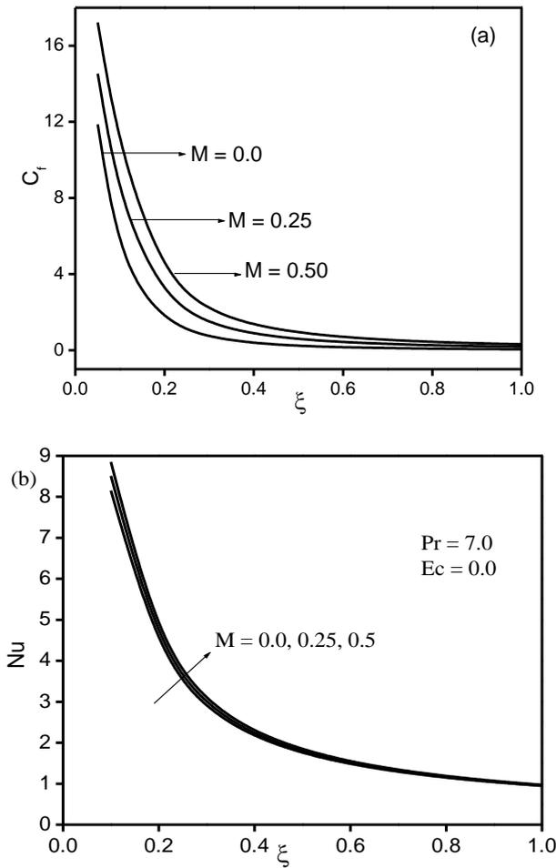
**Fig.2 Effect of Magnetic field on (a) skin friction and (b) heat transfer coefficients**
