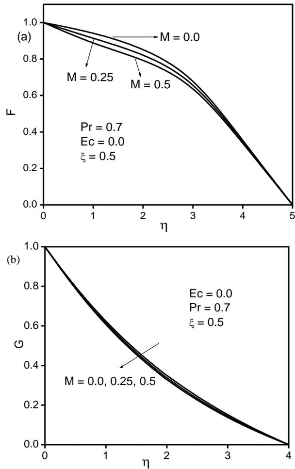
**Fig.3 Effect of Magnetic field on (a) Velocity (F) (b) Temperature (G) profiles**
